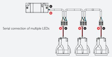
4 Connect luminaire to driver. Place the luminaire into frame.
